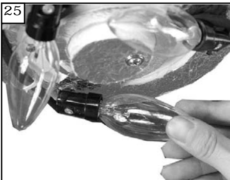
25 Install the 3 x 40 watt incandescent candelabra bulbs.
